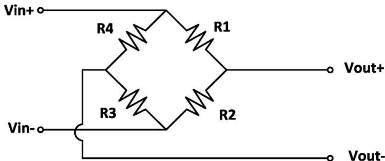
Being  $V_{in}$  the power supply of the bridge or input excitation ( $V$ =Volts) and  $V_{out}$  the output signal ( $mV$ =milivolts).
